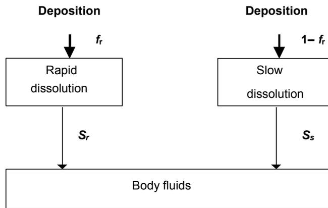
**Figure 6** Compartment model representing time-dependent dissolution, followed by instantaneous uptake to body fluids. A fraction  $f_r$  of the deposit is initially assigned to the compartment labelled “Rapid dissolution”, and the rest ( $1-f_r$ ) of the deposit is initially assigned to the compartment labelled “Slow dissolution”.
