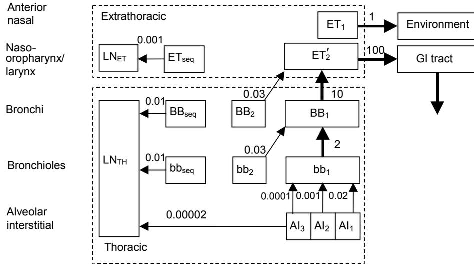
**Figure 5** Compartment model representing time-dependent particle transport from each respiratory tract region in the HRTM. Rates shown alongside arrows are reference values in units of  $d^{-1}$  (Table 1).
