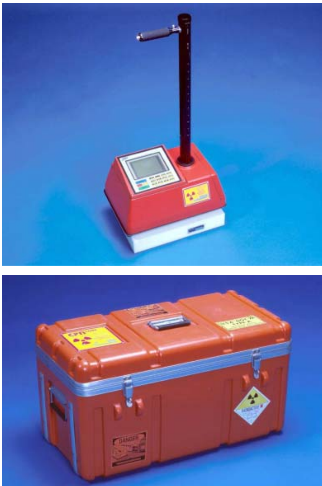
FIGURE 5 Soil density and moisture probe with its carrying case, together forming a Type A transport package
