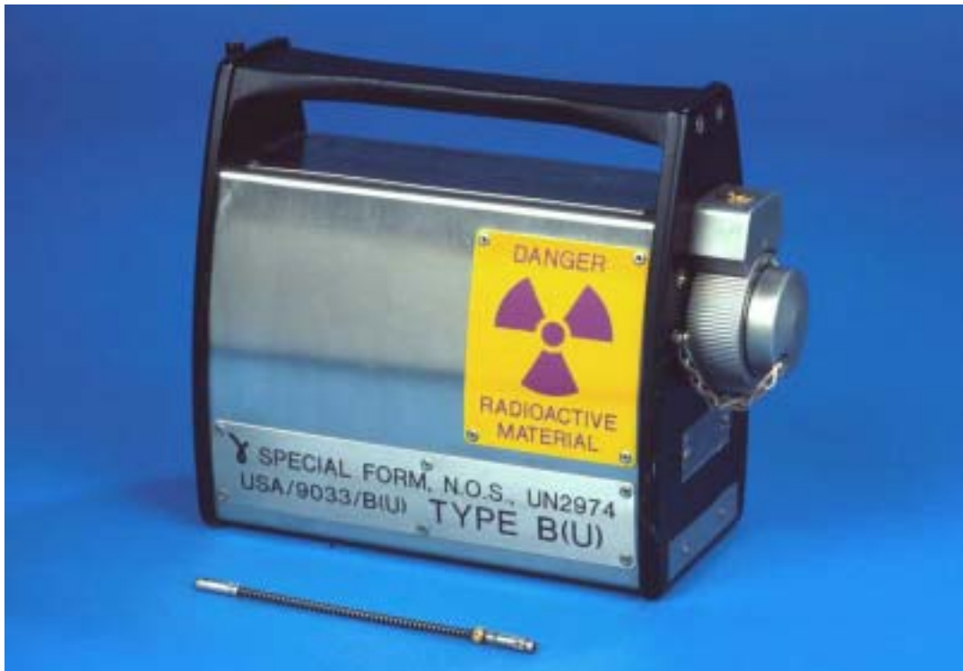
FIGURE 7 Gamma radiography source container – for transport, the source (foreground, left hand end) is locked in the centre of the shielding container
