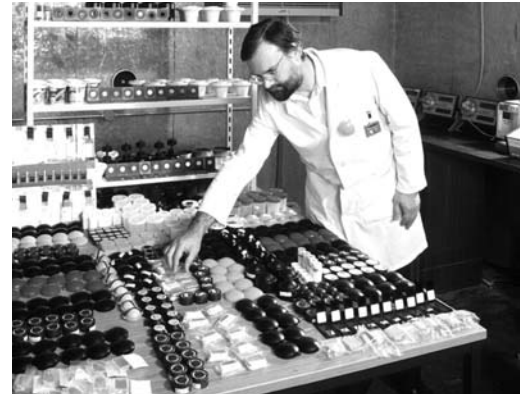
Passive radon detectors exposed during an international intercomparison
