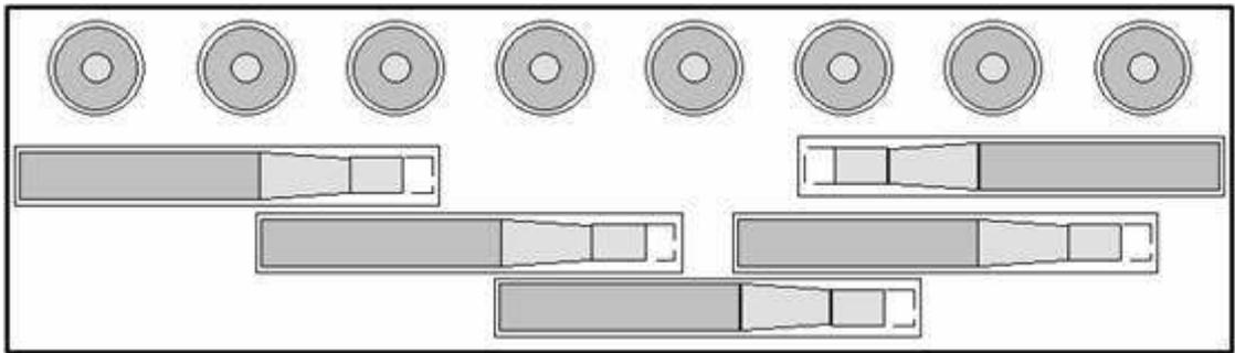
**Figure 2. A schematic showing the arrangement of the Groundhog Synergy detector array in the carbon fibre housing case.** *Reproduced by kind permission of Nuvia Ltd.*
