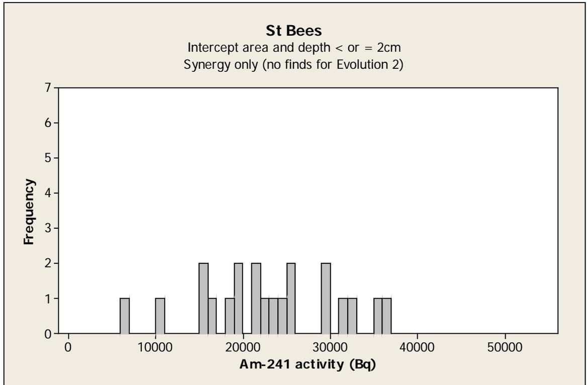
**Figure 15. Numbers of alpha-rich objects found on St Bees beach by the Synergy system. “Overlap” areas only, monitoring campaigns within 1 year of August 2009, objects found at depths less than or equal to 2 cm. No objects were found by the Evolution2 system in the overlap area during this period.**
