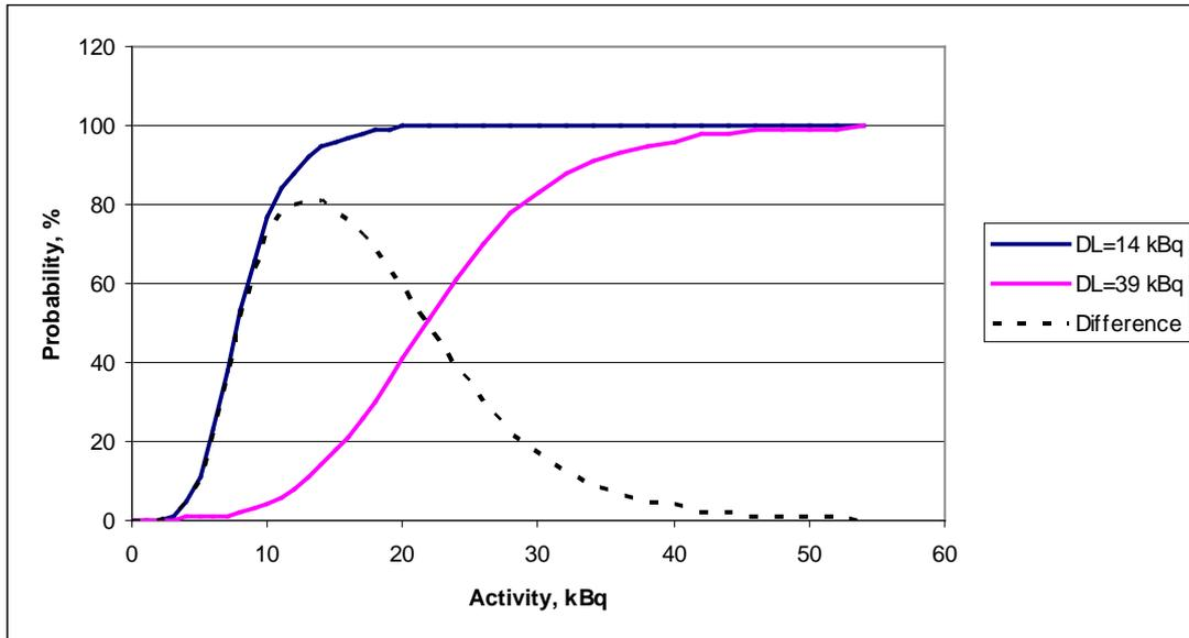
**Figure 3. Object detection probabilities vs. activity of  $^{241}\text{Am}$  for a measurement with detection limits (DL) of 14 kBq  $^{241}\text{Am}$  and 39 kBq  $^{241}\text{Am}$ .**
