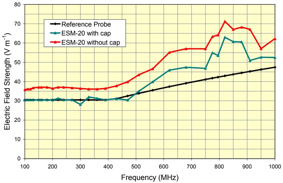
**FIGURE 13** Comparison of E-field reading from a ESM-20 mounted vertically inside a GTEM cell with the reading from a reference instrument
