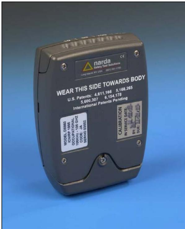
**FIGURE 8 Nardalert XT personal exposure monitor**
