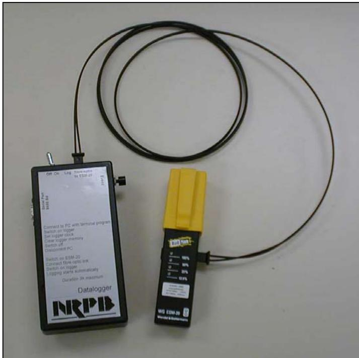
**FIGURE 7** Data logger connected to an ESM-20 'RadMan' personal monitor via a fibre-optic cable
