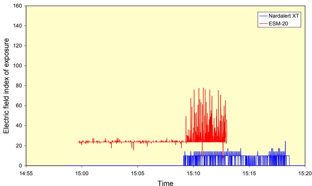
**FIGURE 17 Comparison of electric field strengths recorded by an ESM-20 and a Nardalert XT at a radar site**
