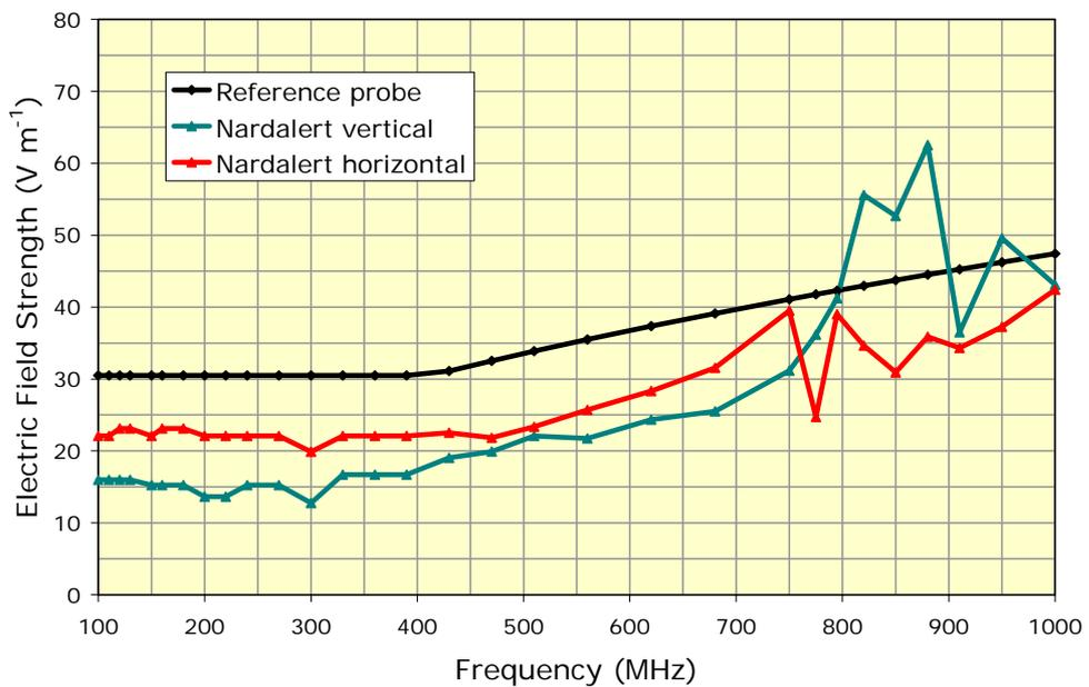
**FIGURE 14** Comparison of E-field reading from a Nardalert XT mounted vertically and horizontally inside a GTEM cell with the reading from a reference instrument
