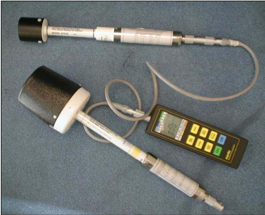
**FIGURE 2** Narda 8712 survey meter with two probes
