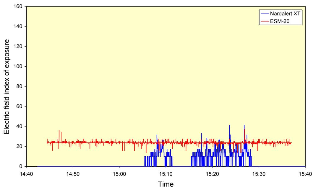
**FIGURE 16 Comparison of electric field strengths recorded by an ESM-20 and a Nardalert XT at a telecommunications site****TABLE 27 Comparison between an ESM-20 and a Nardalert XT at a telecommunications site**
