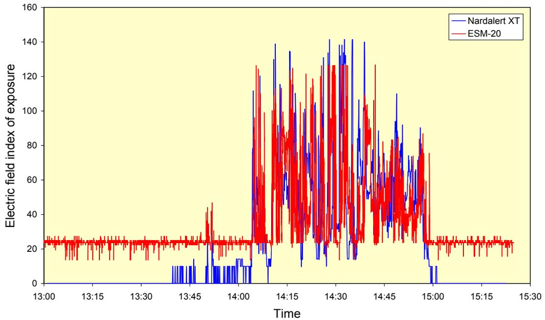
**FIGURE 15 Comparison of electric field strengths recorded by an ESM-20 and a Nardalert XT at a broadcast site**
