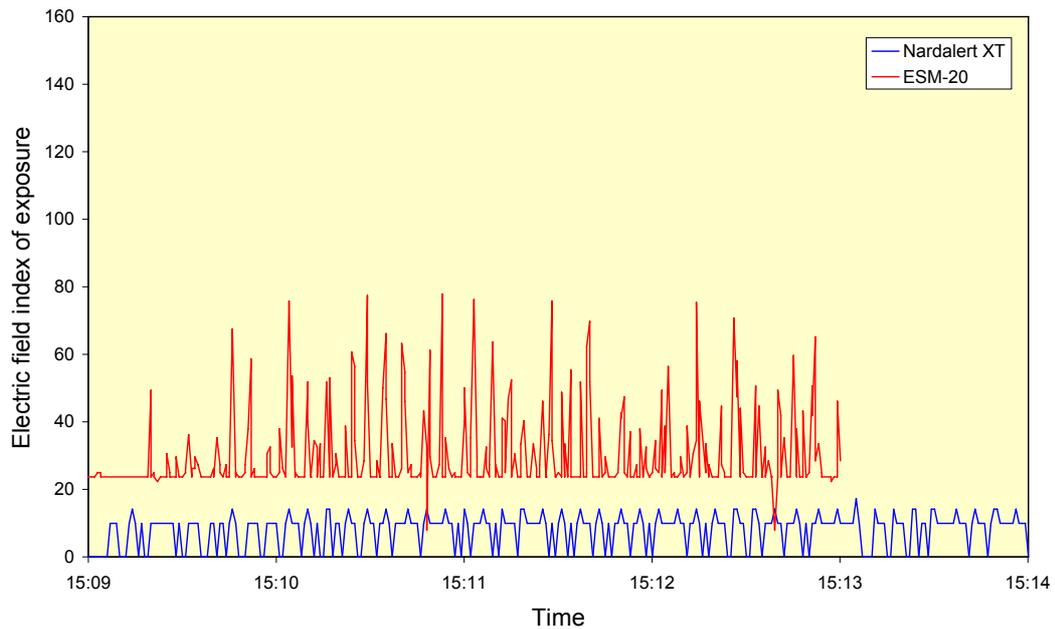
**FIGURE 18 Comparison of electric field strengths recorded by an ESM-20 and a Nardalert XT at a radar site**
